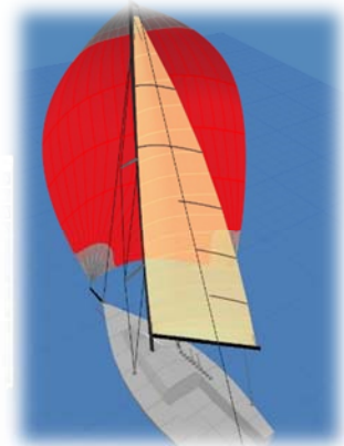
Ease the tack to induce luff projection = deeper angles.
